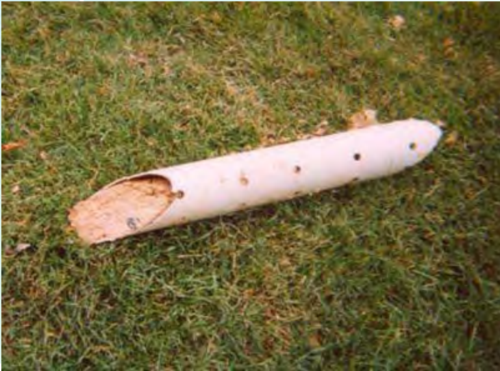
Slotted pipe often block.
