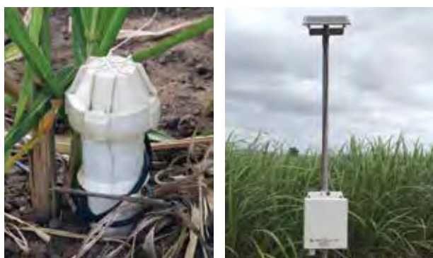
Above: EnviroSCAN probe installed in the field.
