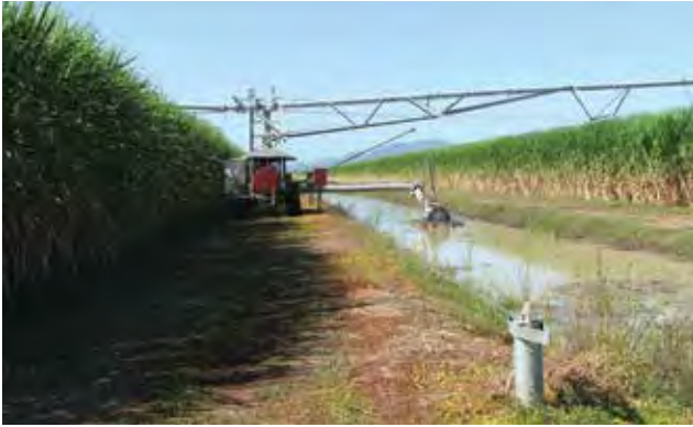
Above: Lateral move irrigator. Photo courtesy of Steve Attard.
