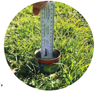
Figure A3-2: Reading application depth in a tuna can
